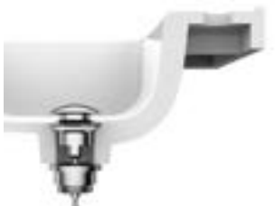
Universal open basin wastes have a fixed open waste cover which ensures water flows from the basin at all times. Suitable for basins without an integrated overflow.
