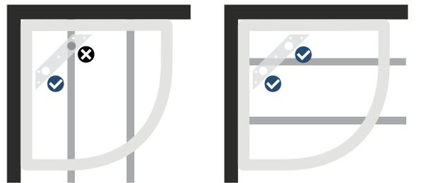
With the unique connect2 design even Quadrant and the Kudos unique Full Curve shape trays have the ability to avoid joists.
